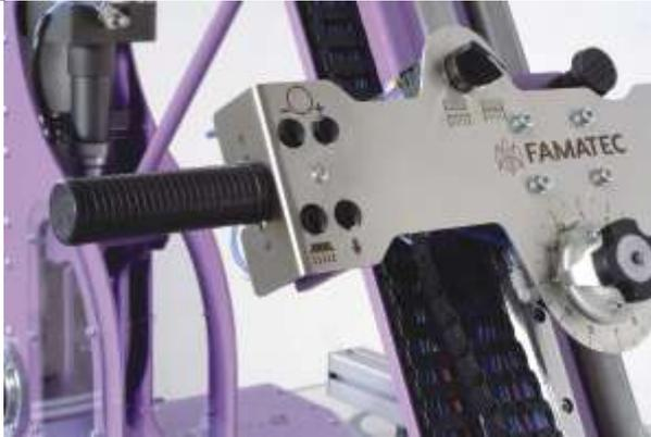
On the console are the controls that adjust the balancing forces to counteract the weight of the product to be handled, and a brake switch that when used, locks the **FAMATEC Friendly** where it is; this allows us to park the equipment at cycle end after use and if necessary carry out further processing on the suspended product.
